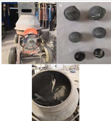
Figure 1: Testing of grinding balls with the mixer petrol driving unit. a) Mixer used in the experiment. b) Tested Grinding balls. c) Grinding mixer in working position
