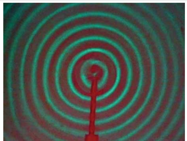
Figure 4: Circular waves on the water surface in the ripple tank.
